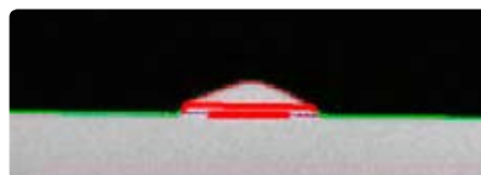
All wafer edges are checked for defects, missing material and glue residues.
